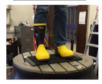
Lab testing identified mats boots and insoles capable of FTV attenuation
